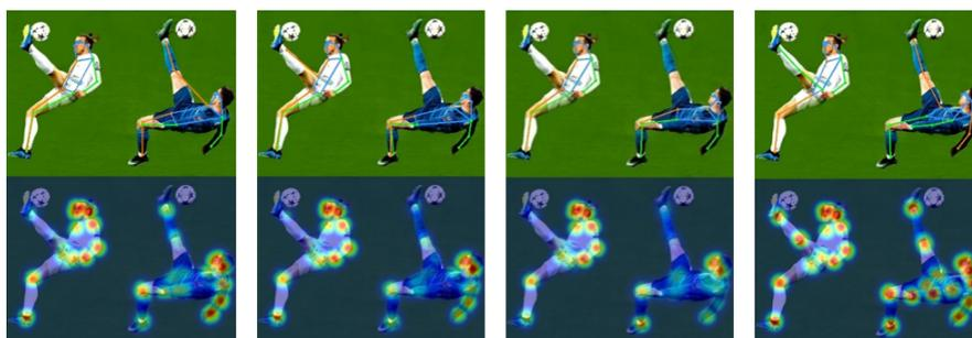
Figure 11. Comparison results of human pose estimation and heat map under human pose distortion using Faster-RCNN as a human detector. (a) MobileNetV2. (b) ShuffleNetV2. (c) Lite-HRNet. (d) Lite CSW-HRNet.
